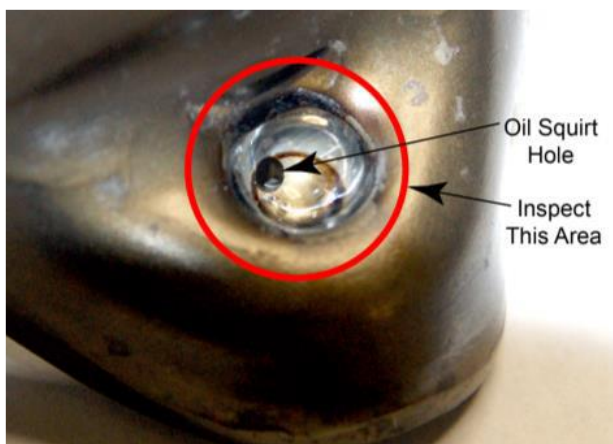
Picture 9 – Pushrod socket side of the rocker arm
