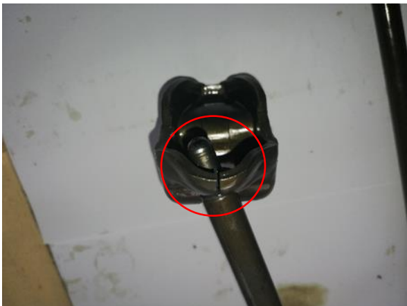
Picture 4 – Damaged exhaust rocker arm
