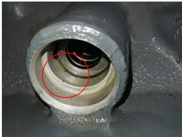
Picture 5 – Surface damage of the canal of the hydraulic lifter
