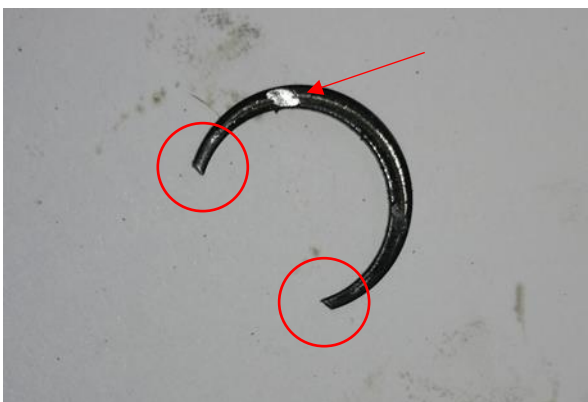
Picture 6 – Cracked safety ring
