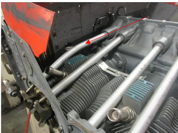
Picture 2 – Bent pushrod of the intake valve lifter
