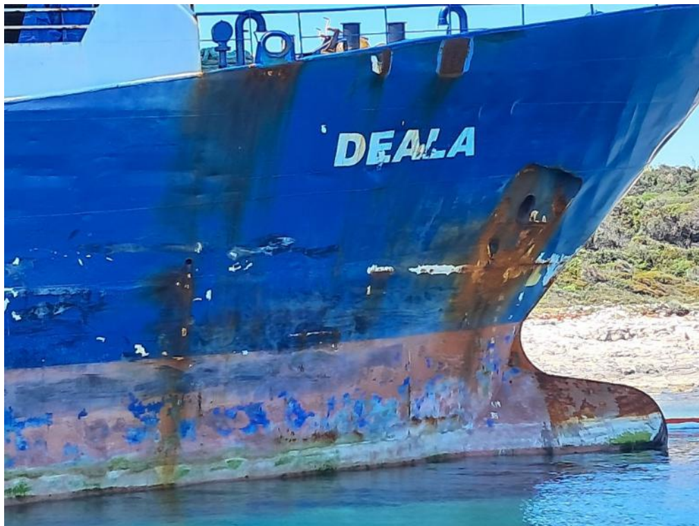
Figure 2. Cargo Ship Deala, after the accident, lost starboard anchor (source: AIN)
