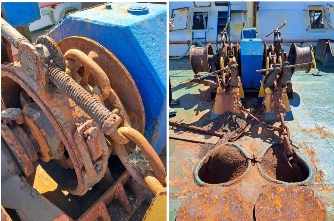
Figure 5: Cargo ship Deala after the accident – the brake on the starboard windlass (source: AIN)
