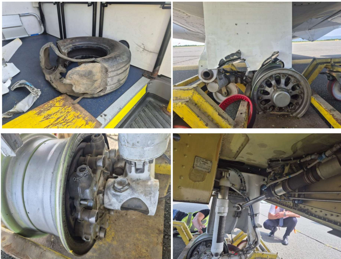
Picture 7 - the tyre, wheel rim, brake and other components of the left landing gear
