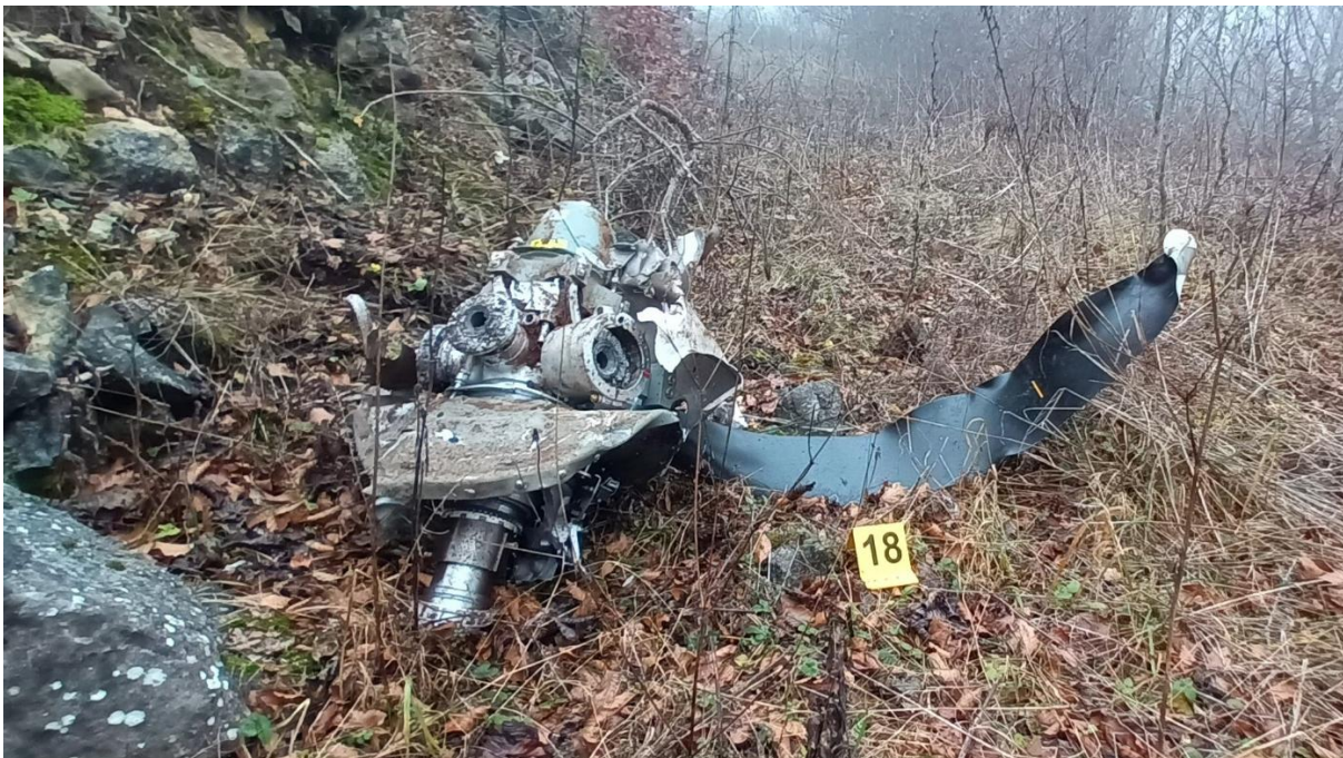
Figure 5 – hub with one propeller blade
